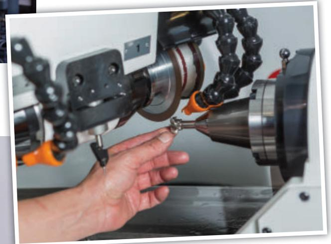
The new tool grinding machine can grind tools from 1 to 100 mm in diameter and up to 255 mm in length.
