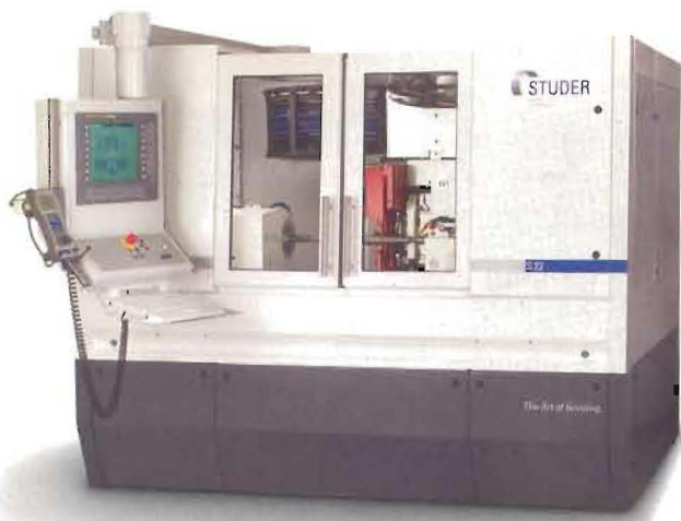
The Studer S22 can be used with one or multiple grinding wheels to complete a part with different features in one clamping.
