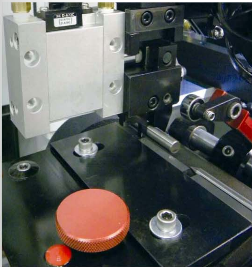
A gripper loads the part onto the workstation.
