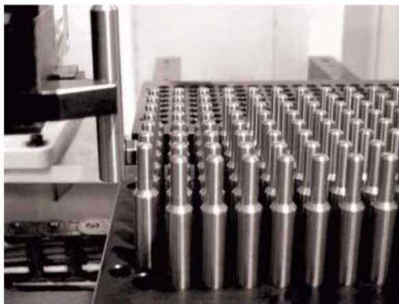
Another gripper unloads the part into a pallet.
