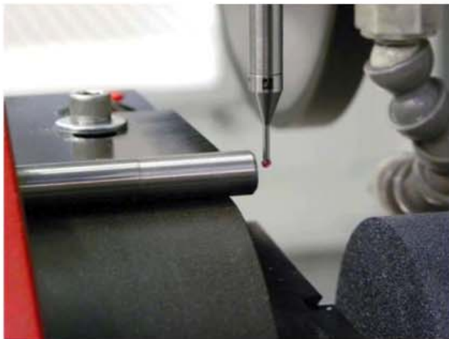
The grinder is equipped with a probe to measure the length of the parts
