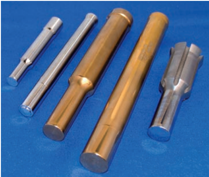
Hi-Quality Carbide grinds precision carbide punches that feature high length-to-diameter ratios. Punches range in size from 0.300"-dia. by 4" - long to 1.25"-dia. by 13"-long. They require a significant amount of precision contour grinding, must meet size tolerances of 0.000,3" – 0.000,5", and surface finish requirements of 2-3 \mu\text{in. } R_a prior to hand polishing.
