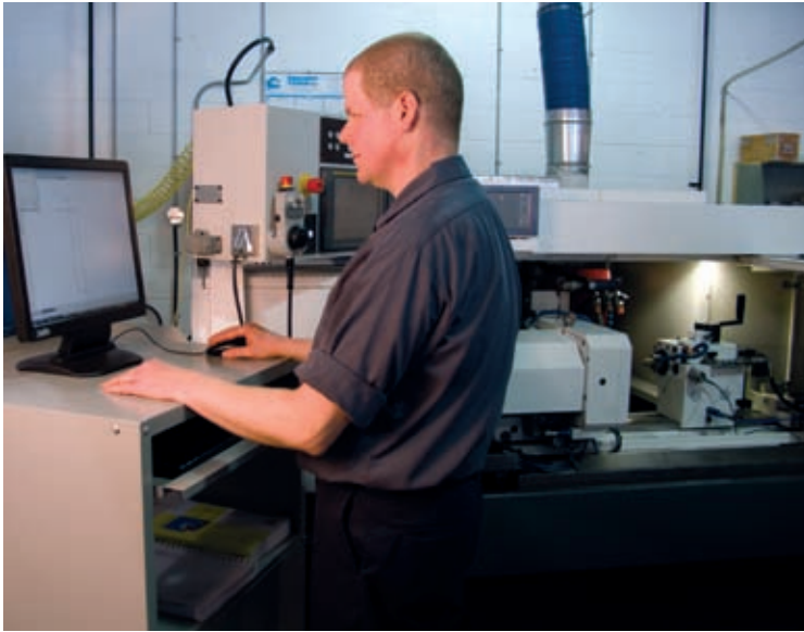
An operator uses StuderGRIND software running on a PC to define the many dimensions of a profile to be ground. The PC is linked to the S33 grinder with an Ethernet cable, enabling easy program transfer. The operator can even make a drawing and set up contours for the next job while the machine is running.
