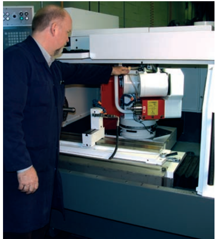
Mark Roman says it is an easy process to switch back and forth between OD and ID grinding. "The ID wheel is behind the OD wheel, and you can lift up the wheelhead and manually swing it around to the ID position."
