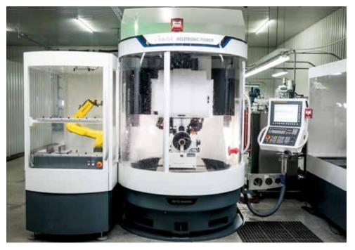
Robotic part loading and unloading allows unattended machine operation.
